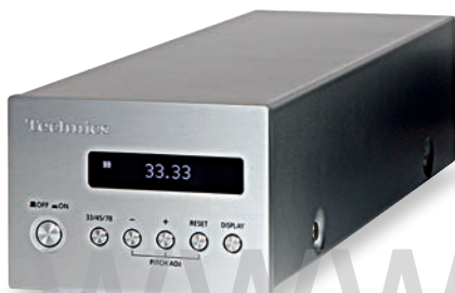
ABOVE: Dedicated outboard PSU delivers a synthesised feed for 33.33, 45 and 78rpm (with ±16% of adjustment). Speed is selected on the deck itself
